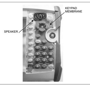
Figure 18. Keypad Membrane
