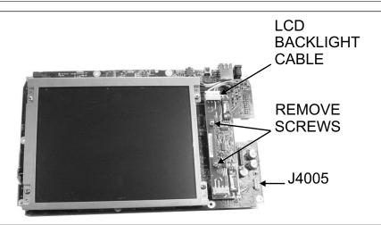
Figure 16. LCD Backlight PCB Removal and Replacement
