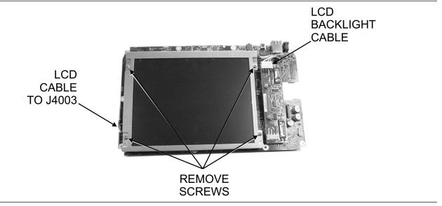
Figure 15. LCD Assembly Replacement
