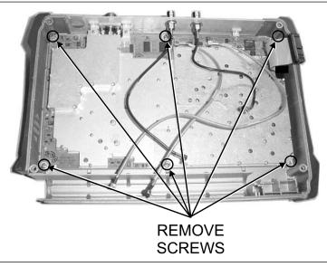
Figure 14. Spectrum Analyzer Module Removal
