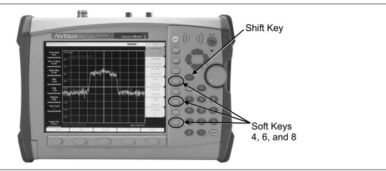
Figure 1. MS2721A Spectrum Master Service Mode Key Sequence
