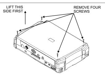
Figure 9. Removing the Cover Screws
