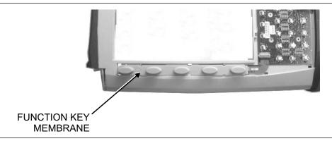
Figure 20. Function Key Membrane
