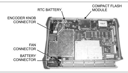
Figure 13. Main PCB Assembly Replacement
