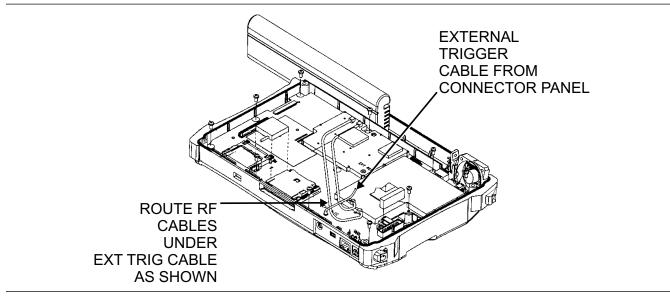
Figure 11. Cable Routing Diagram
