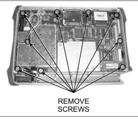
Figure 12. Main PCB Assembly Mounting Screws
