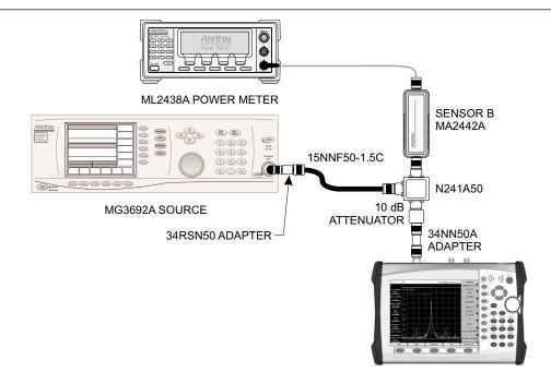
Figure 3. Frequency Level Accuracy Test Setup
