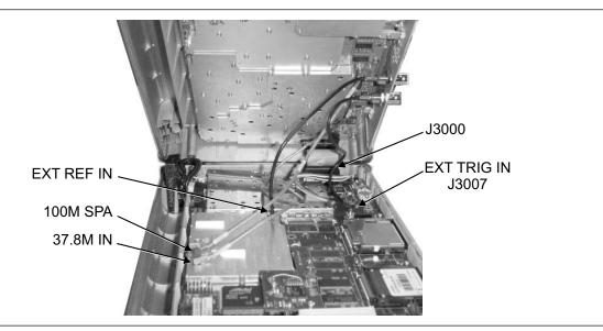
Figure 10. Front Panel Assembly Removal and Cable Connections
