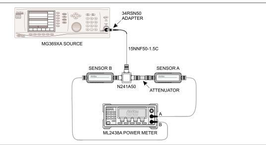
Figure 2. Level Accuracy Across Frequency Component Characterization Test Setup
